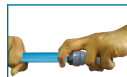
Step 5: Inserting the Tubes into fitting
